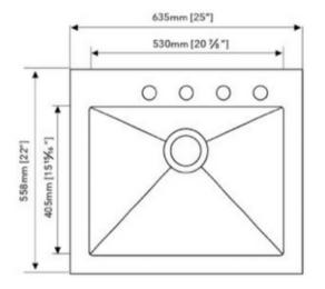
Undercoated and Sound Pads 3-1/2" Drain Opening
